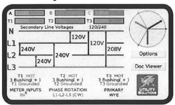
secondary, modify phase orientation, explore multiple secondary voltages and different transformer settings. It simulates back-feeding and reduced capacity services so users learn and practice real-world troubleshooting.
