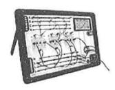
Utility Solutions Inc. has a new three-phase distribution simulator specifically designed to teach transformer banking to lineworkers. The updated Load-Trainer II Transformer Simulator combines a physical wiring environment with powerful computer simulation. The new one-piece design is very portable and weighs just 16 pounds. Several new features came directly from training
